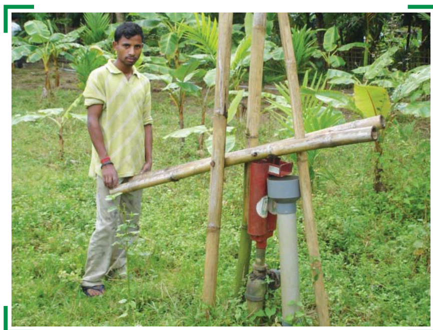
Low cost treadle pump being used for cultivation of banana in Betanipam village, Sisiborgaon block, Dhemaji district under the ICAR supported project 'Live Better with Floods'
