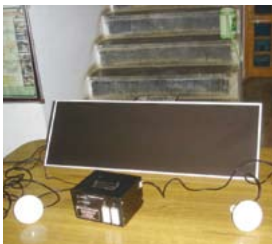
The LED-Lamp Unit comprising a solar panel, a charging-cum-controlling unit and two lamps
